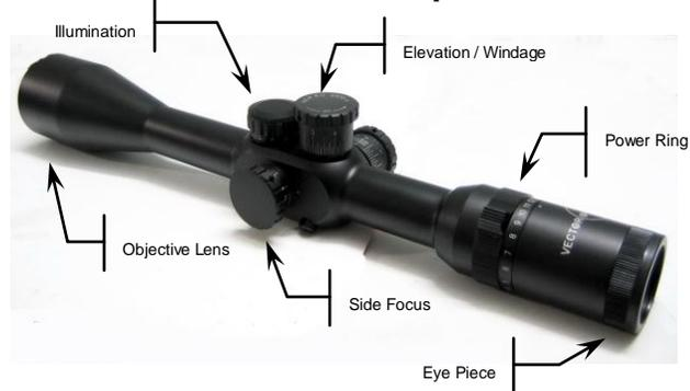
**FFP Brief Introduction:** The scopes fit the reticle in the first focal plane. The reticle increases its size when change the magnification from low to high. The advantage with telemetric reticles (like rangefinder & Mil-dot etc) is that the target image and distance between dots remains constant even when changing magnification.
